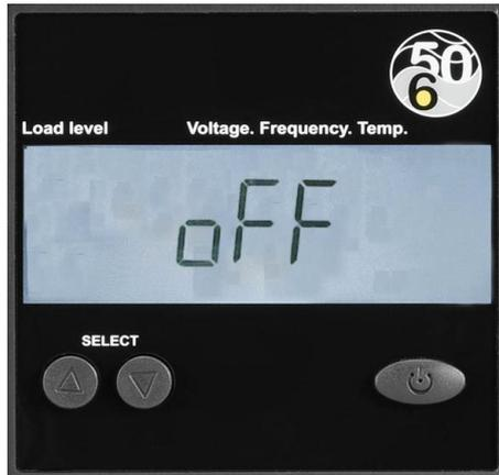
**4.4 Change the Output Voltage and Frequency:** To push the two selection buttons,  $\triangle$  and  $\nabla$ , at the same time for 3 seconds until the LCD display begins to blink.
