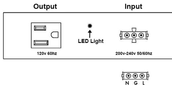
**3-Pin Locking Connector Set: Input (4 of the Most Commonly Used Plug Type Power Cords)**
